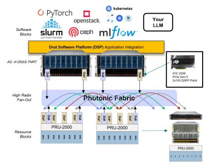
Traditional servers often end up underutilized, leading to the need for expansion. Drut and Supermicro tackle this challenge with an innovative expansion system based on an OSI layer 1 photonic fabric, using a unified orchestration system, that avoids heavy costs and allows you to focus on LLM deployment.
