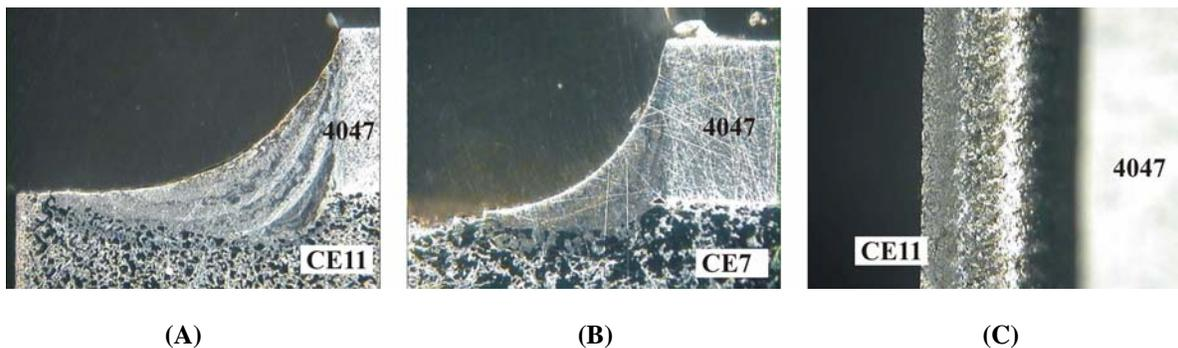
**Figure 4** Welds completed with lid positioned 0.04” from the alloy edge. (A) CE11, with 50% silicon content (B) CE7 with 70% silicon content (C) Plan view of CE11 seam showing crack free weld.
