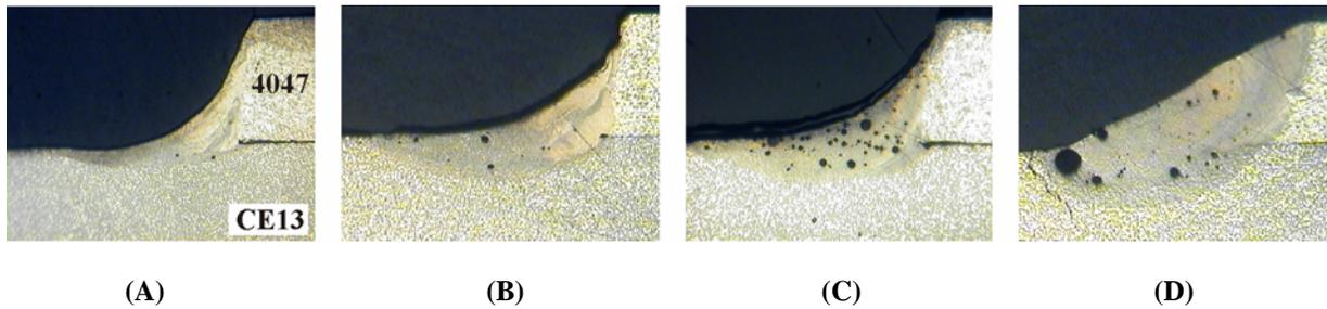
**Figure 2** Cross sections of seam welds in CE13 (Al-40%Si) at various conditions. (A) 8kW, 1ms, 10 Hz, 0.1"/s. (B) Offset into Al-Si alloy; 5kW, 1ms, 17 Hz, 0.15"/s (C) Insufficient or excessive gas pressure (D) 2kW, 20ms, 10 Hz, 0.1"/s.
