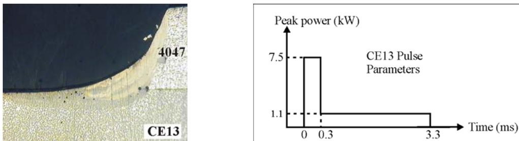
**Figure 3** Cross section of CE13 weld with the pulse shape used.
