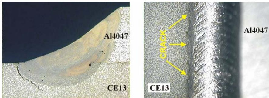
**Figure 1** Cross section of an un-optimized seam weld indicating the location of crack, that occurs outside of the weld in the heat affected zone of the Al-Si. A top view of the weld shows the crack clearly running the length of the seam
