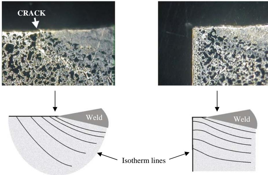
**Figure 5** Micrographs of the a CE11, 50% silicon alloy, weld edge at x300 magnification, both for away from edge and at edge welds. The schematic sketches show the isotherm lines and how the edge weld modifies these to prevent the stress field adjacent to the weld.
