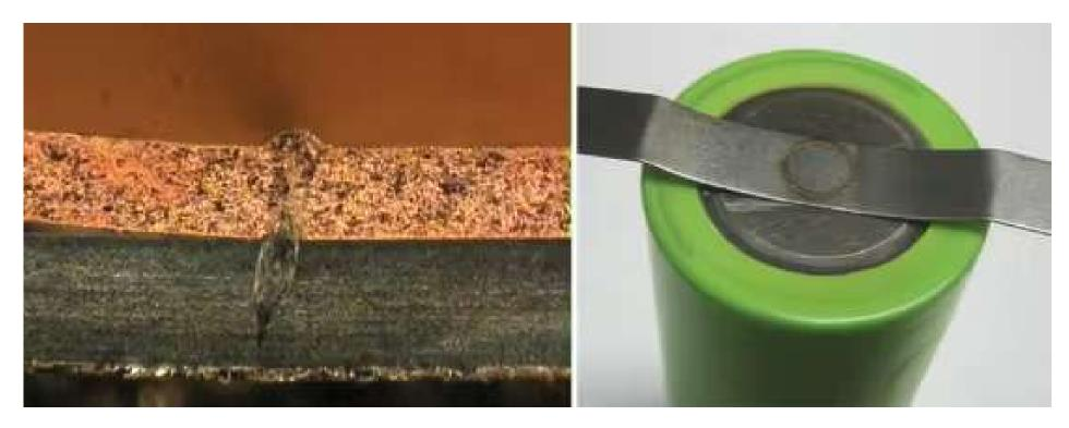
When welding a tab to a terminal, the general rule of thumb is that the tab should be thinner than the can terminal thickness. As the can thickness decreases, the tab usually must be 50 percent of the can thickness for a safe essing window that provides weld strength and conductivity without penetrating the can.
