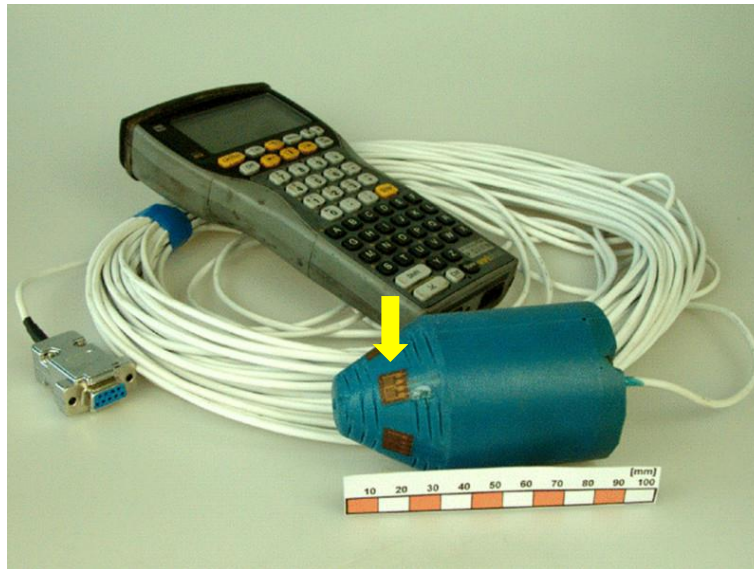
Figure 5 Cone Tool showing cable and readout unit. Strain gauges shown about the snout of the tool (arrowed).
