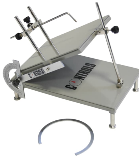
Figure 13 Example of tilt test apparatus (Image source: https://controls-group.com/it/product/dispositivo-di-prova-del-coefficiente-di-rugosita-del-giunto/ )
