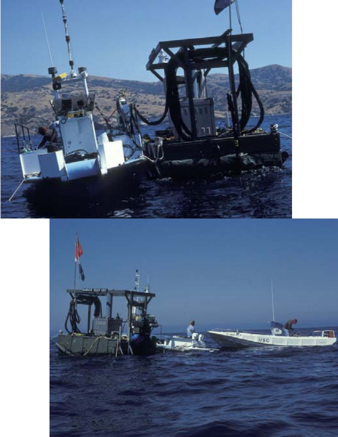
Figure 2. Support barge with hot water and air supply.
