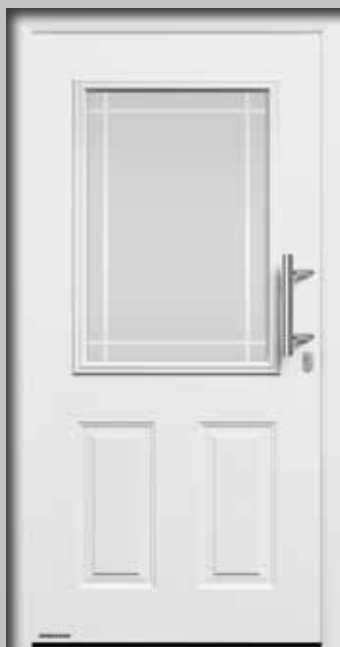
Style 430 Stainless steel handle HB 14-2 on steel infill, triple-pane insulated glass, exterior laminated safety glass, centre sand-blasted float with clear stripes, interior clear laminated safety glass, U_D -value up to approx. 1.0 \text{ W}/(\text{m}^2\cdot\text{K})^*
