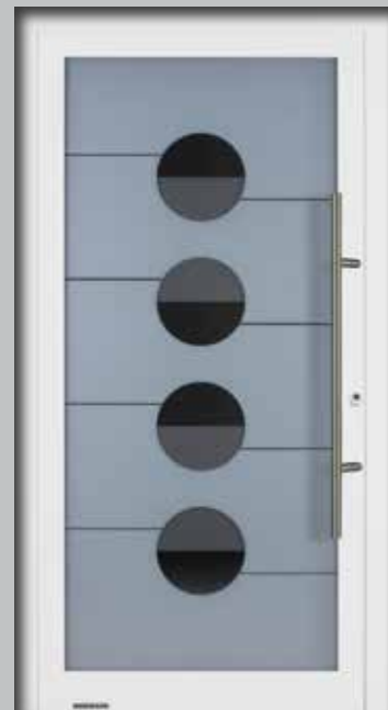
Style 100 / MG 114 Stainless steel handle 38-1, design glass, exterior: matt laminated safety glass with 4 clear circles and 8 clear stripes, 6 mm, centre: single-pane safety glass, Stopsol grey, with 4 matt semi-circles, interior: clear laminated safety glass, U_D -value up to approx. 1.6 \text{ W}/(\text{m}^2\cdot\text{K})^*
