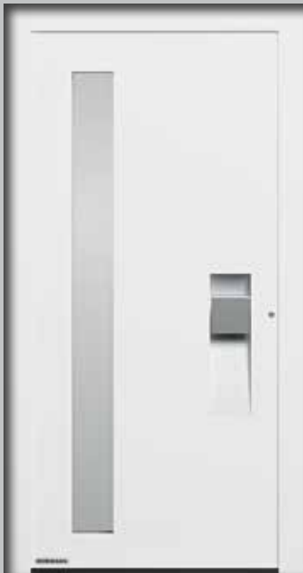
Style 314 Flush-fitting stainless steel handle as standard, recessed grip in door colour as standard, matt float ornamental glass, quadruple thermal insulation glass, certified low-energy house door, U_D -value up to approx. 0.57 \text{ W}/(\text{m}^2\cdot\text{K})^*
