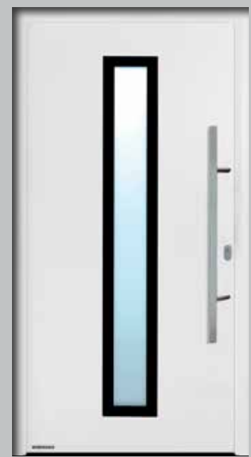
Style 600 ■ NEW from 1.7.2017 Stainless steel handle HB 38-2 on steel infill, with surface-mounted glazing: triple-pane insulated glass, exterior laminated safety glass, centre sand-blasted float, interior clear single-pane safety glass
