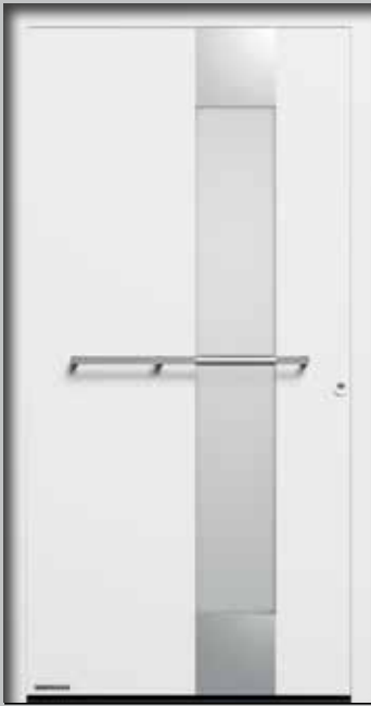
Style 555 Stainless steel handle HOE 910, stainless steel embellishment, Reflo design glass with sand-blasted design, triple thermal insulation glass, U_D -value up to approx. 0.9 \text{ W}/(\text{m}^2\cdot\text{K})^*
