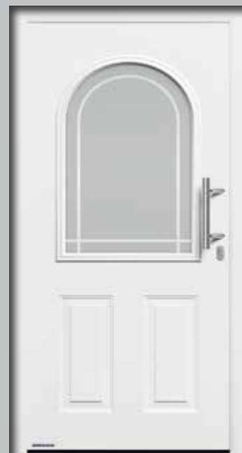
Style 450 Stainless steel handle HB 14-2 on steel infill, triple-pane insulated glass, exterior laminated safety glass, centre sand-blasted float with clear stripes, interior clear laminated safety glass, U_D -value up to approx. 1.0 \text{ W}/(\text{m}^2\cdot\text{K})^*
