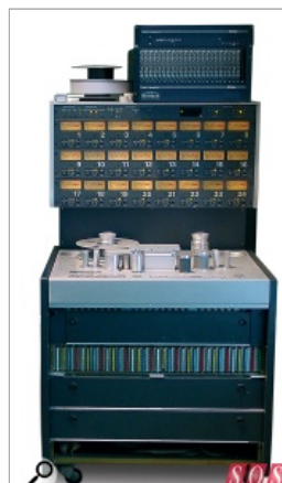
Multitrack Tape Machine & Tape: Tape drive, EQ and bias settings, tape type and machine electronics will all affect the sound, as do the cumulative effects of tape imperfections when tracks are bounced down to create space for overdubs.
