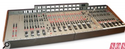
Mixing Desk: May include valves, transformers, and inductor-based EQ, or may be a passive mixer with make-up gain amplifiers.
