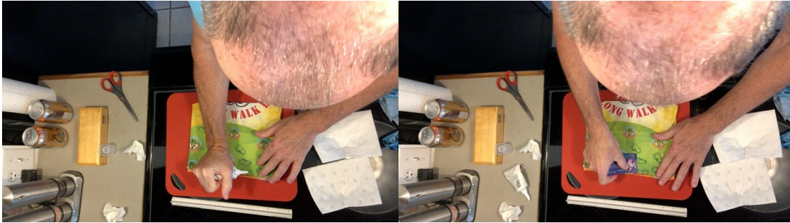
Figure 7: Forming Thin Silicone Nose Seal, Then Flattening
