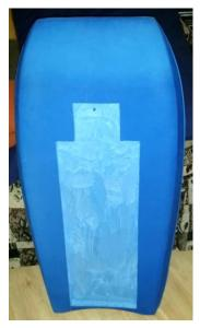
At the time of making my first board, I did not have a router and ended up using a very sharp carving knife to fillet out the foam, so if you don't have the listed tools, normal kitchen utensils can work too to slice out the cavity.
