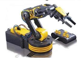
(Same day shipping if ordered by 4 P.M (EST) Monday - Friday Command the Robotic Arm Edge for multiple movements and functions • Robotic arm gripper opens and closes • Movement included radial wrist motion of 120°, an extensive elbow range of motion 300°, base rotation of 270°, base motion
