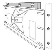
Level Wall Plate and mark location of holes. (Six Holes on Plate)
