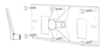
Drill 5/16" pilot holes in center of wall stud in marked areas.
