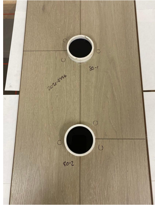
Figure 31: 80-Hour T-Seam at commencement of test
