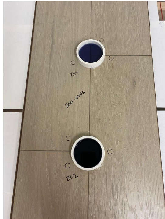
Figure 15: 24-Hour T-Seam at two-hour mark
