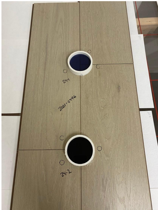
Figure 12: 24-Hour T-Seam at commencement of test
