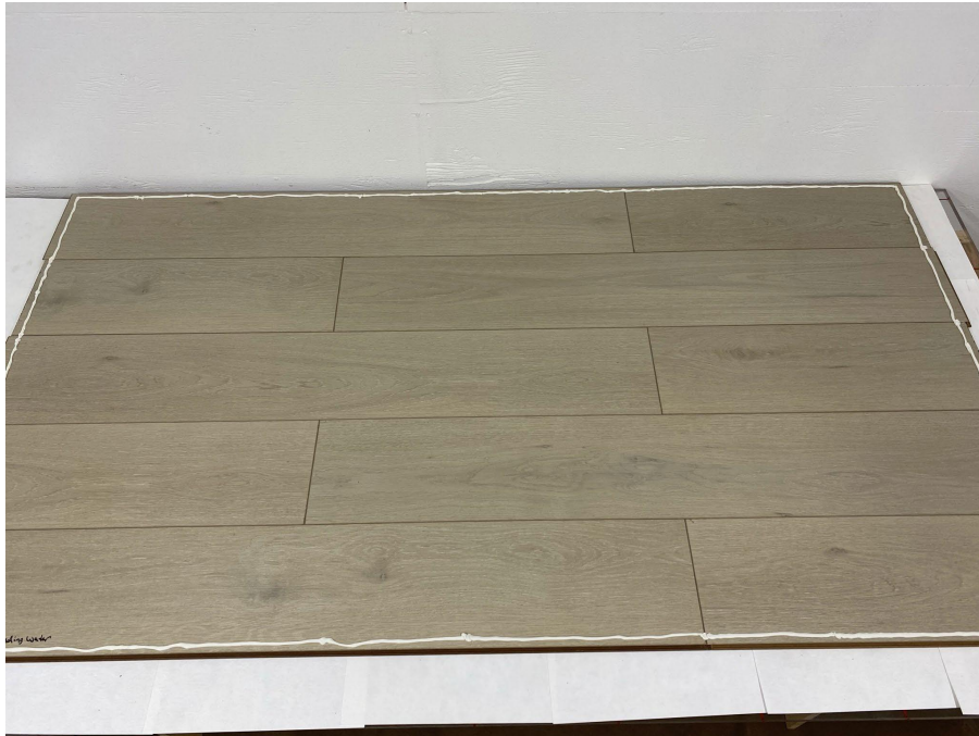
Figure 1: 30-Hour Standing Water Test Assembly prior to addition of water
