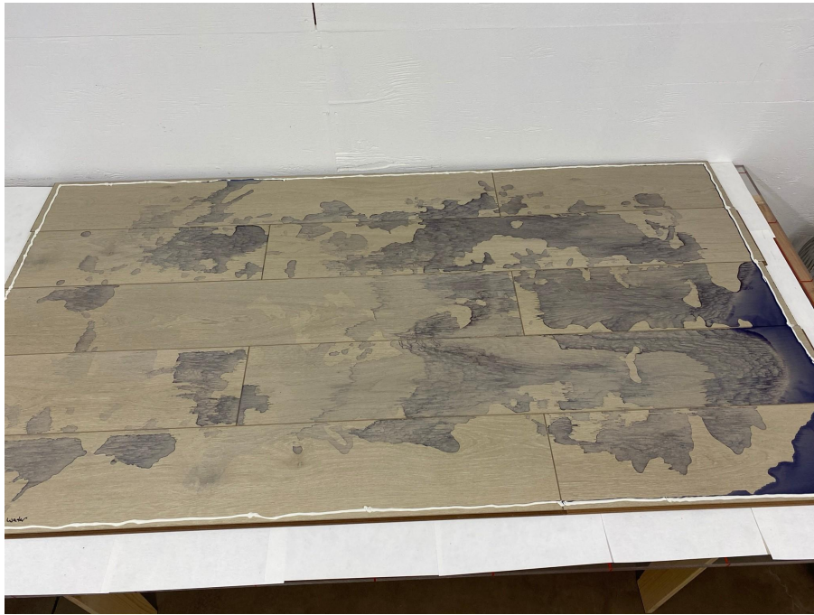
Figure 9: 30-Hour Standing Water Test Assembly at the 24-hour mark
