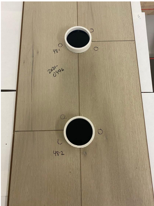
Figure 24: 48-Hour T-Seam at two-hour mark
