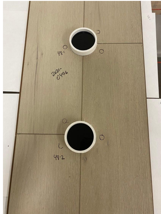
Figure 21: 48-Hour T-Seam at commencement of test
