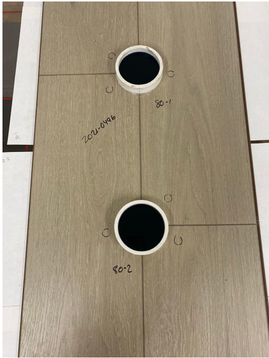
Figure 34: 80-Hour T-Seam at two-hour mark
