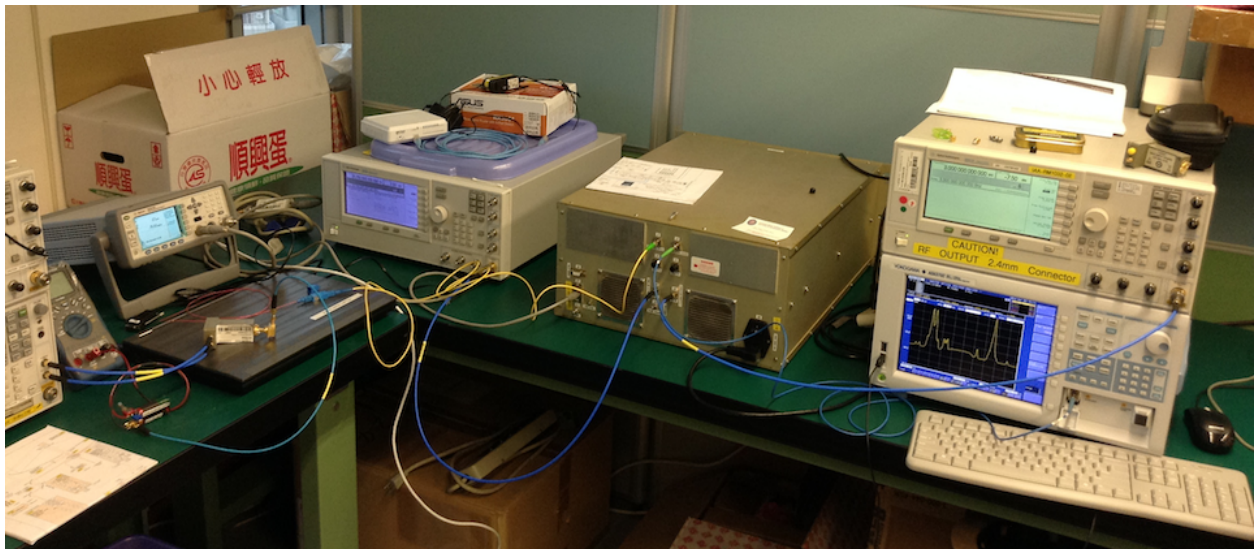
Fig. 1 LORTM Test Setup. Rear panel view of LORTM (center). OSA on right shows optical spectra for 100/106 GHz. Ref. 1 = 25.75 GHz, Ref. 2 = 3.00 GHz.
