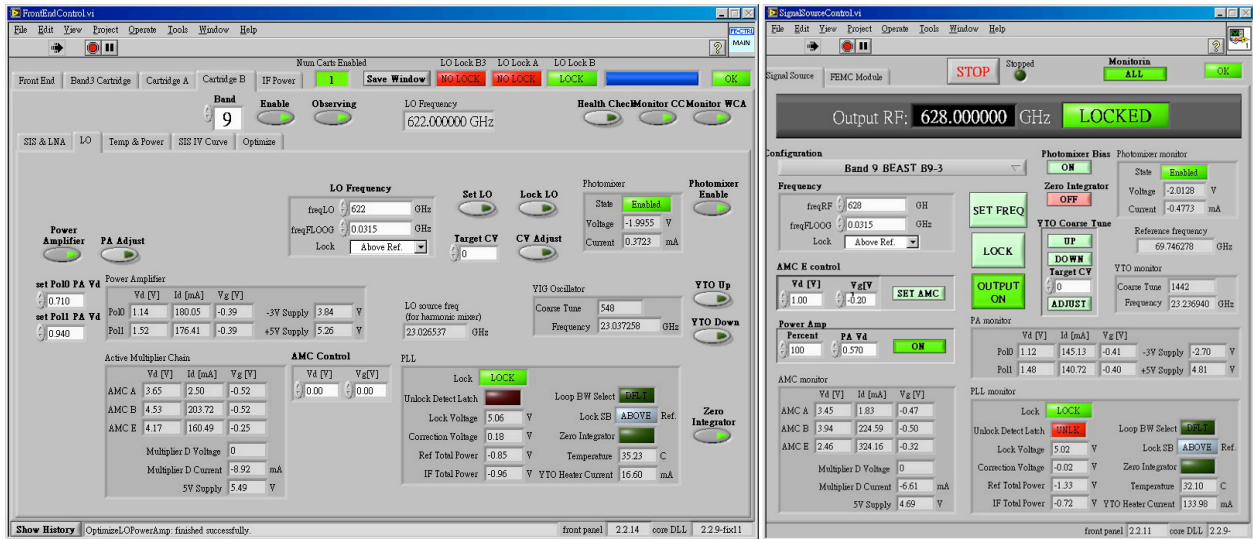
Figure 30 Screen shots Front End Control and Signal Source Controls for 622/628 GHz FE test.
