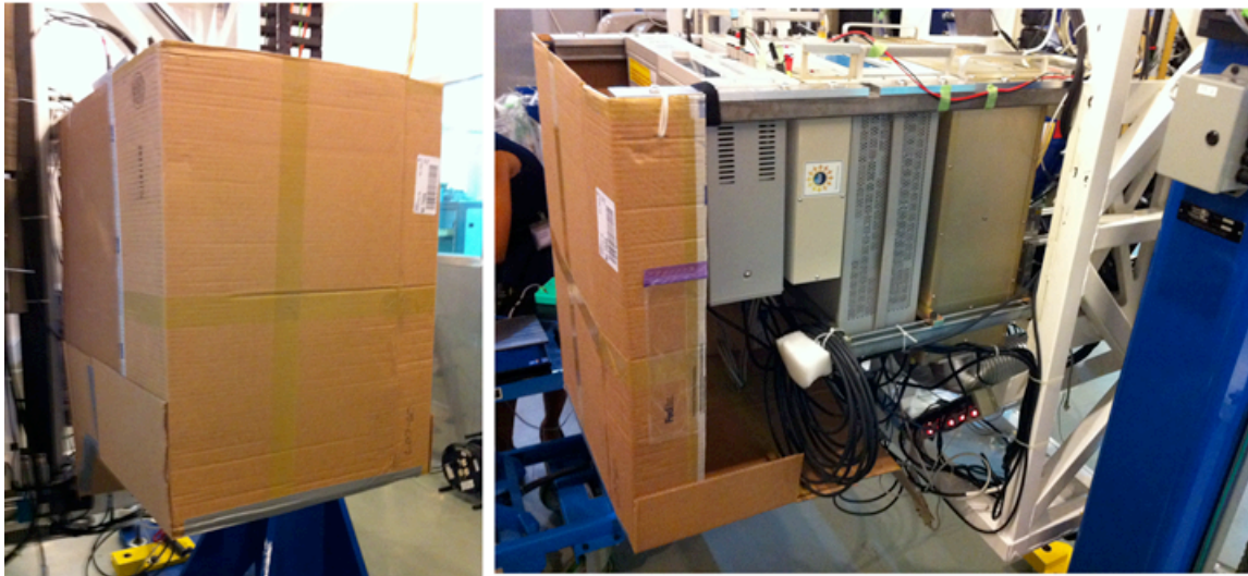
Figure 38 Removable cardboard shroud around tilt rack at 0 degree elevation. The shroud covers the entire left side, about 75% of the rear panel area, and it opens on the right side. At 60 and 90 degrees the bottom portion faces the rear wall. Air channels up through the rear bottom portion and out the top opening. This photo was taken prior to the moving of the Extra IF Plate chassis (2 nd from left).
