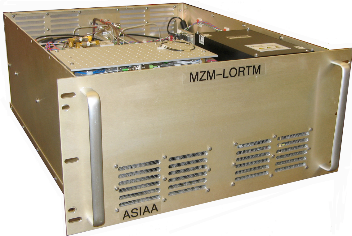
Figure 7 Oblique view of completed MZM LORTM, July 2011. The physical dimensions of this unit, including the front panel rack mounting holes, are identical to the baseline TeraXion LORTM unit. Note the air exhaust vents located toward the bottom of the front panel.
