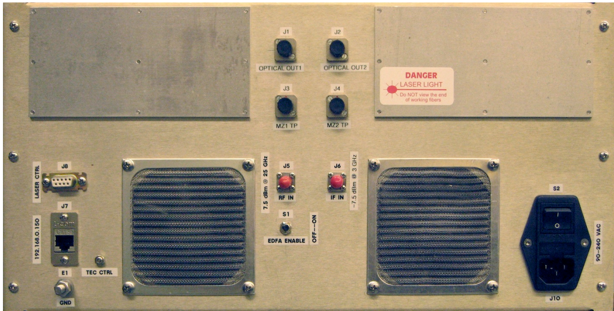
Figure 9 Rear panel. All inputs and outputs are via the rear panel. Note the blocked exhaust air vents at the top to keep the upper deck isolated from the ambient air temperature variations. Only the lower deck is convection cooled and critical elements from the upper deck are conduction cooled through the aluminum deck plate.
