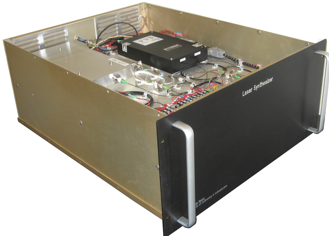
Figure 1 Oblique view of completed MZM Laser Synthesizer, July 2010. Chassis is rack mountable, 19 x 22 x 8.75 inches, fully EMI compliant, total weight of 42 pounds (19 kg) with covers installed.
