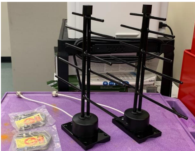
Figure 5. Log periodic antennas with gain of 9.1 dBi and beam width of 35 degrees.
