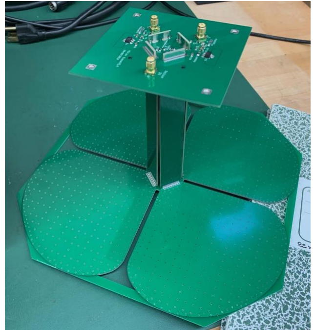
Figure 6. Clover leaf feed consists of two pairs of opposing petals forming a pair of orthogonal dipole antennas. The radio signals collected by the 6-meter dish is focused onto the feed.
