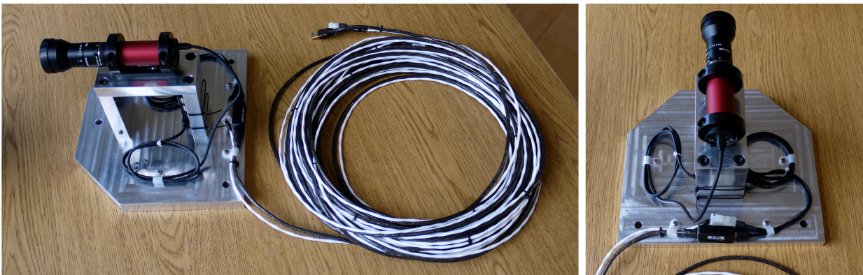
Fig. 4 – Photo of completed interconnects to SBIG camera (only one 20-meter extension cable shown). Note the USB hub is wire tied to the right vertical support plate and barely visible in the left photo. Both the USB (black) and +5V power (white) extension cables are wire tied together.
