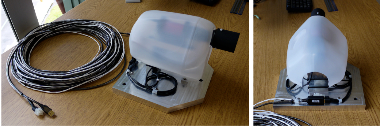
Fig. 5 Photo of completed camera assembly with cover and lens hood. The cover is held to the assembly with two 8-32 Phillips head screws. The lens hood is held to the lens with three white plastic blade head screws.
