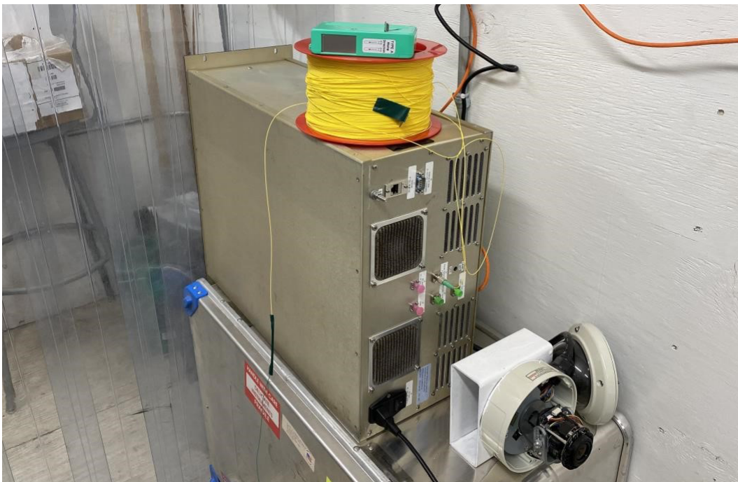
Figure-3. Rear view of the Laser Synthesizer located within the Maser House. The yellow spool on top consists of 200 meters of single-mode fiber with FC/APC connectors on each end. Though this fiber is not protected by a jacket it may be used temporarily to test the effectiveness of the beacon on the tower.
