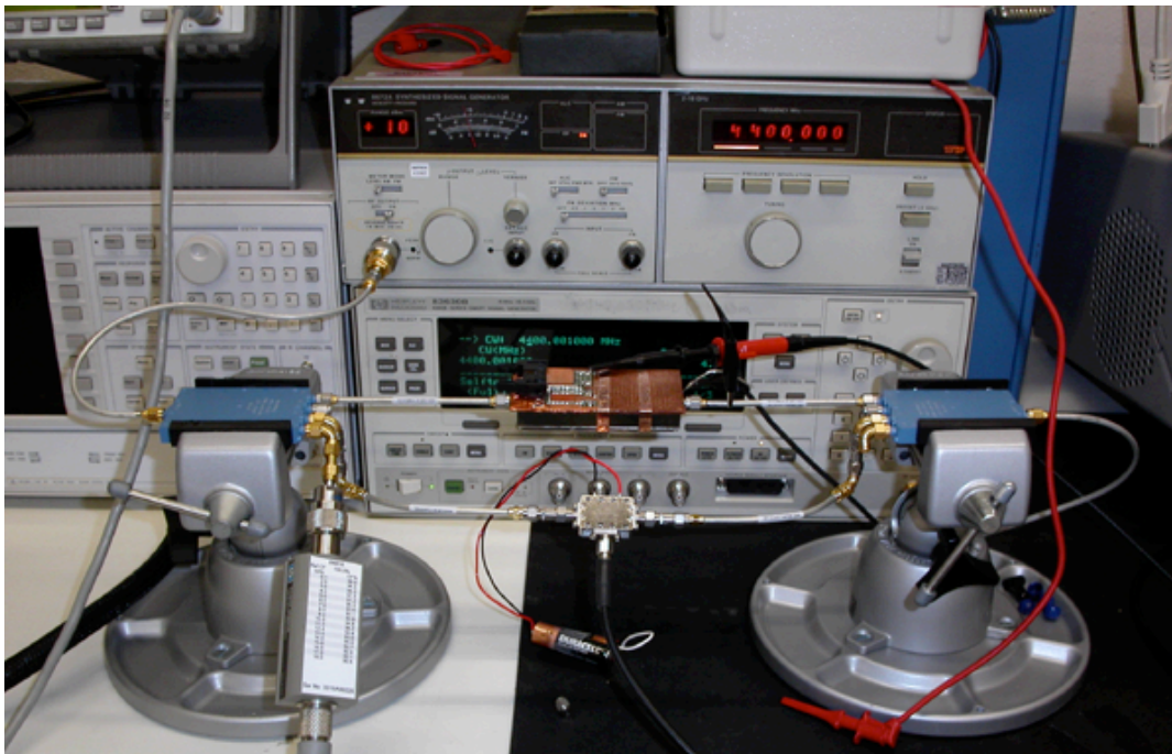
Figure 7 – Photo of Phase Test Setup
