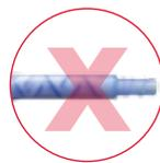
The mixing chamber of the ColorWise nozzle will change from clear to blue when cold chemical is sprayed through it. Stop spraying and ensure proper chemical temperature to avoid off-ratio foam.
