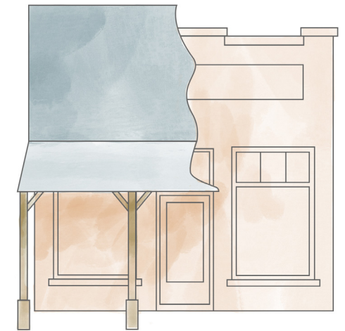
The original parapet has been covered by a false wood front.
