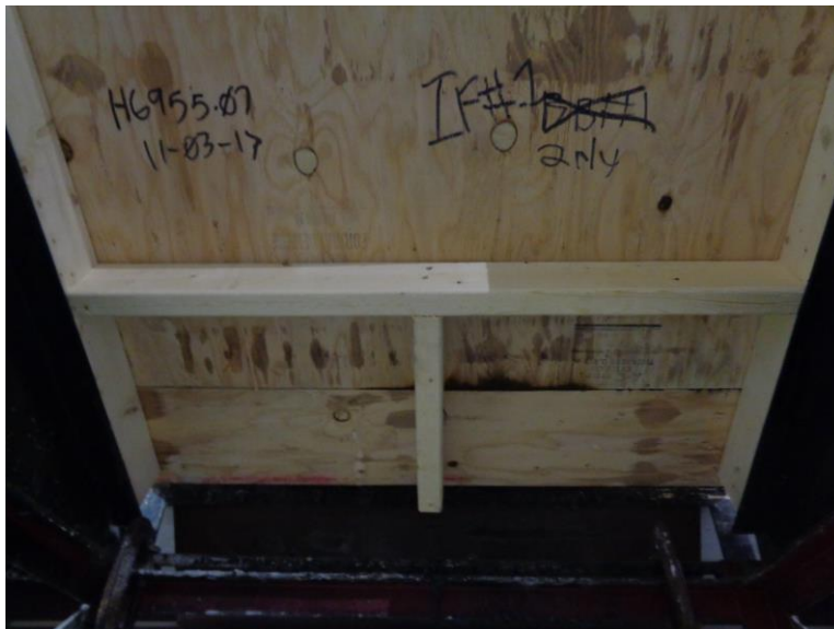
Photo No. 6 Assembly #1 Intermittent Flame #1 Underdeck During Test
