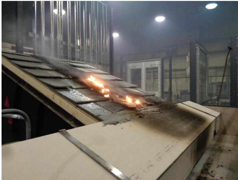
Photo No. 5 Assembly #1 Intermittent Flame #1 During Test
