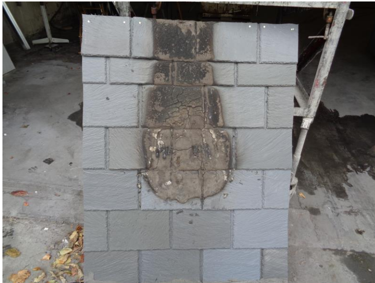
Photo No. 38 Assembly #2 Burning Brand #3 Post Test
