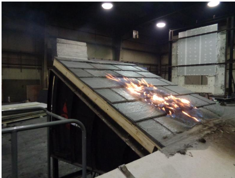
Photo No. 16 Assembly #2 Intermittent Flame #1 During Test
