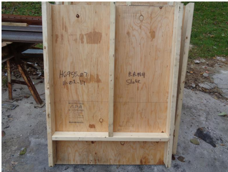
Photo No. 42 Assembly #2 Burning Brand #4 Underdeck Post Test
