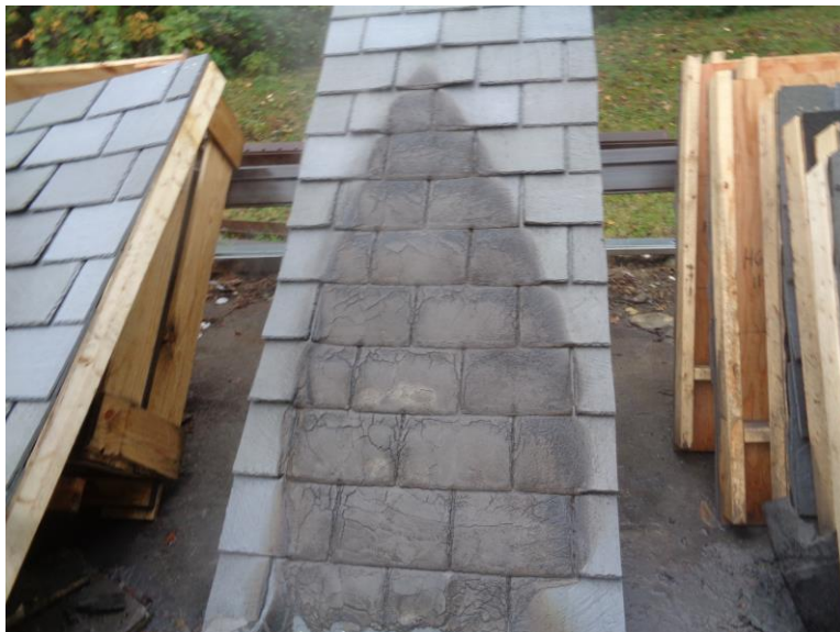
Photo No. 26 Assembly #2 Spread of Flame #2 Post Test
