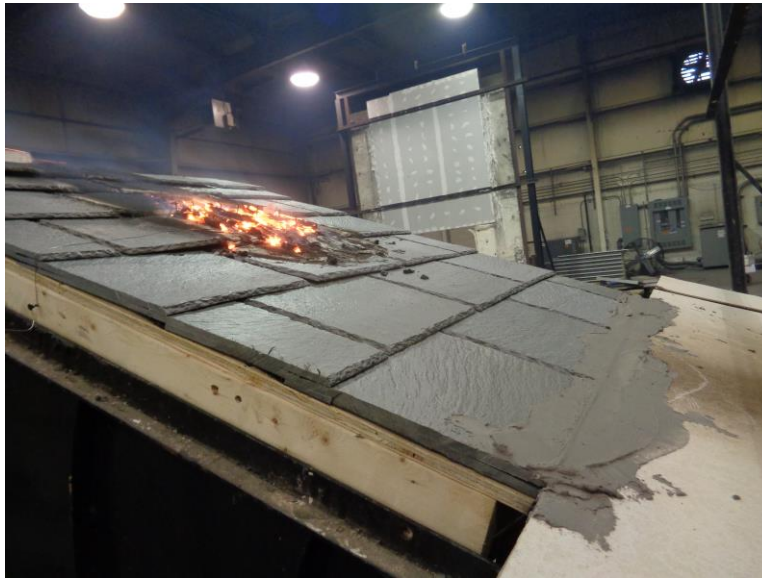
Photo No. 37 Assembly #2 Burning Brand #3 During Test
