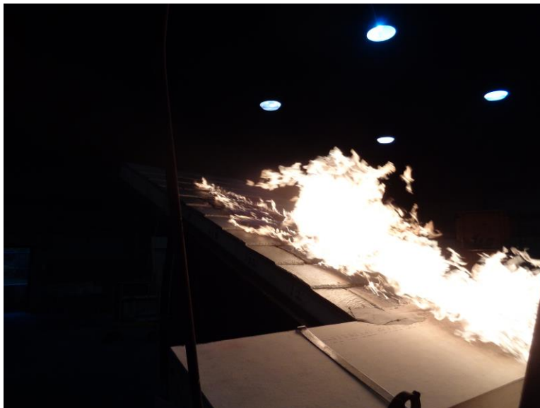
Photo No. 22 Assembly #2 Spread of Flame #1 During Test
