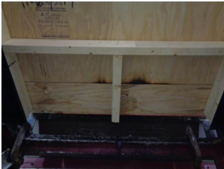
Photo No. 10 Assembly #1 Intermittent Flame #2 Underdeck During Test
