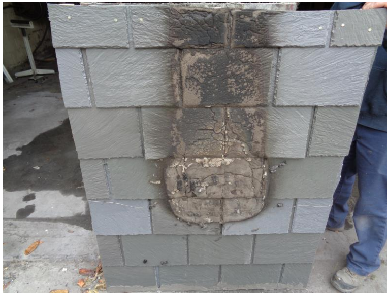
Photo No. 41 Assembly #2 Burning Brand #4 Post Test
