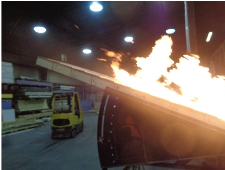
Photo No. 25 Assembly #2 Spread of Flame #2 During Test
