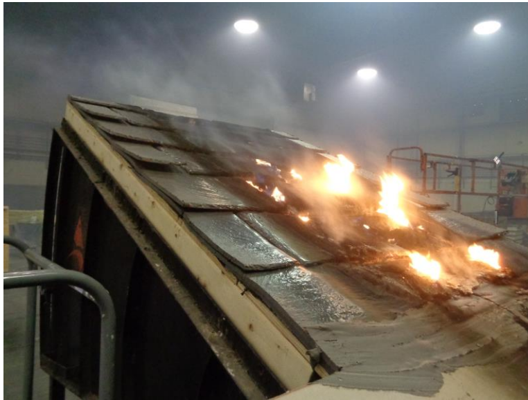
Photo No. 9 Assembly #1 Intermittent Flame #2 During Test
