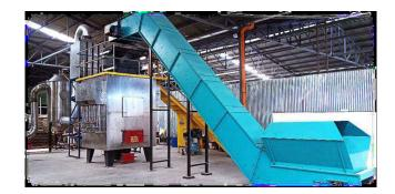
The MSW to Ash Base solution will use NON-SEGREGATED MUNICIPAL WASTE and convert it into <u>Ceramic Ash</u> that <u>can be sold to the Cement Factories for use in Burners</u>. The metals and glass in the MSW need to be separated from the Ceramic Ash.
