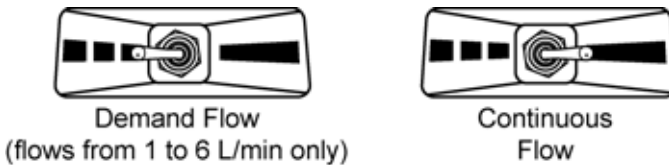
Figure 17: Continuous/Demand Flow Switch
