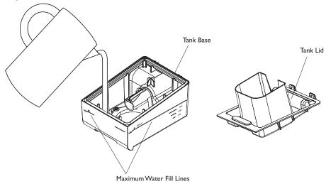
**CAUTION:** Use only room temperature distilled water in the tank. Do not put any chemicals or additives into the water. Possible airway irritation or damage to the water tank may result.
