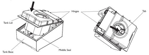
**Note:** If the lid does not close easily onto the base, separate the two parts, reassemble the tank, and inspect it again. **CAUTION:** Do not fill the water tank above the maximum fill line. Damage to the humidifier or therapy device may occur. If the water tank is overfilled, water may leak out of the tank inlet (located on the back of the tank) when installing the tank lid.
