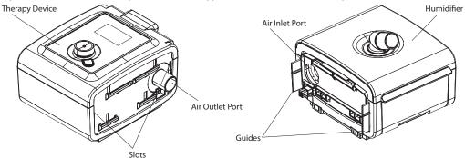
4. Simply press the two units together until they snap into place. Make sure that the therapy device and the humidifier are completely seated against each other.
