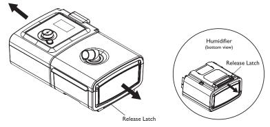
3. If you will be using the therapy device without the humidifier, reattach the side cover to the therapy device.
