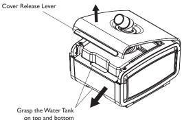
3. Press the tab in the hole on top of the tank in toward the front of the tank. Gently remove the tank lid from the tank base and set aside. Empty any remaining water from the base of the tank.
