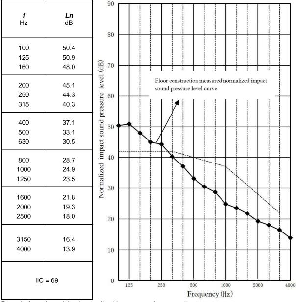
Remark: *L<sub>n</sub>* as the weighted normalized impact sound pressure level
