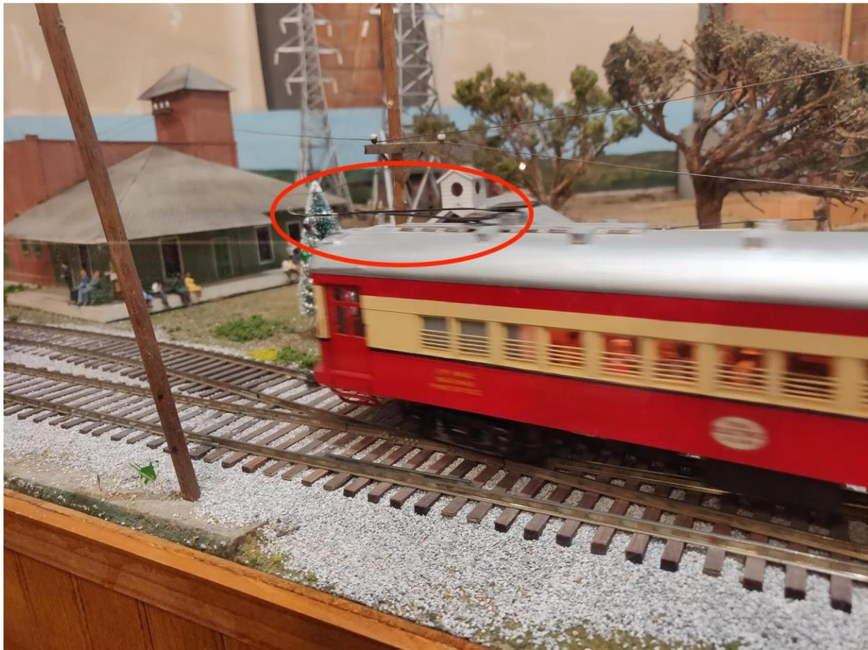
The Interurban Railway ran on **direct current (DC) electricity**, which means energy only flowed in one direction, from the Plano substation to the trolley wires. Trains connected to the wires with a **trolley pole**, which is circled in **red** in the image above. As long as the trolley pole was connected to the wires, the train received electricity and was able to move down the railroad track.
