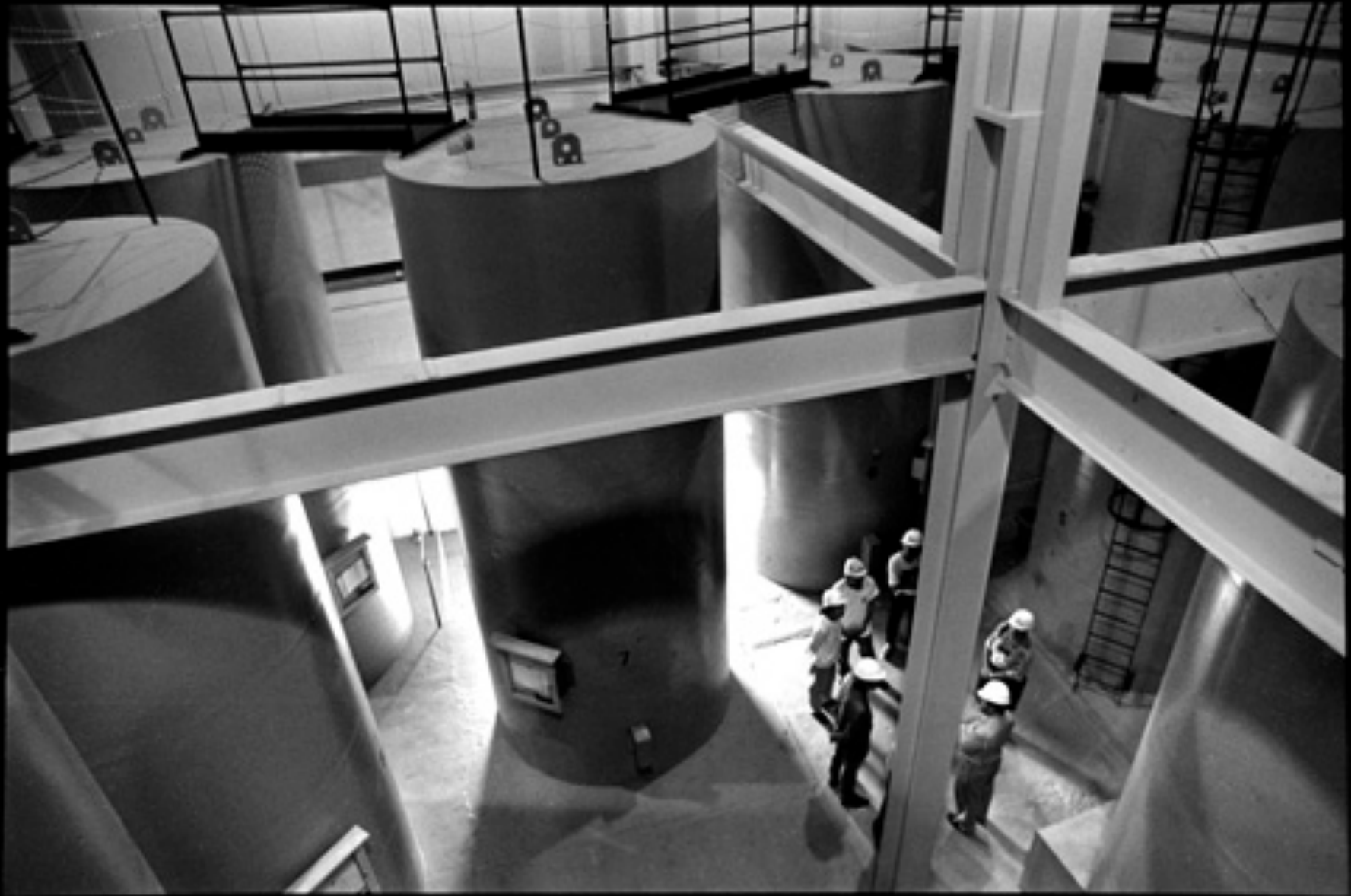
After 10 years in the pool, CANDU spent fuel is put into air-cooled "dry storage" containers.
