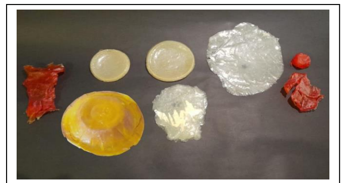
Fig 4. Bioplastic of the desired shape obtained based on the shape of the mould.
