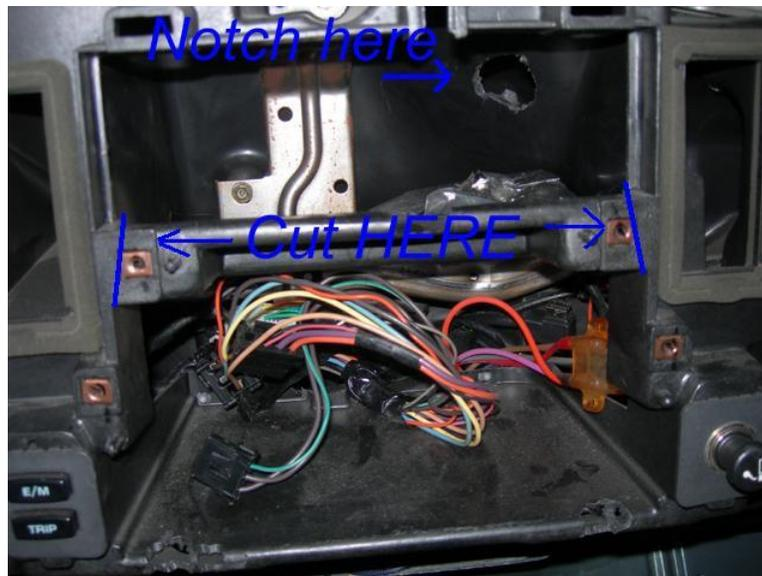
Depending on the depth of your head unit, the vent tube may need to be notched and resealed. See the “Notch Here” in the above pic.
