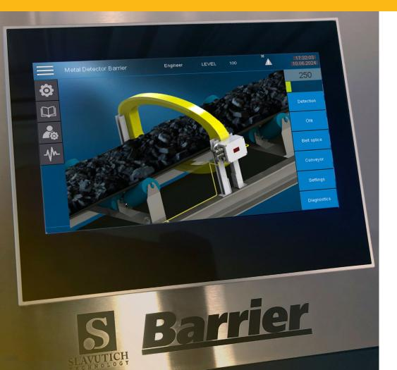
The 3B409E control module is a high-performance real-time system equipped with an integrated multi-touch display for maximum visualization and convenient control of the metal detector. The module supports Ethernet, RS-485, CAN, and optionally Profinet connections. It also features user access control, event logging, and real-time visualization of the metal detector's primary data.
