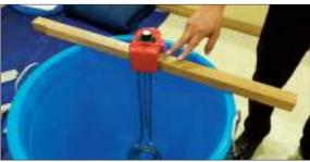
Use 3kw heater for 500 L (132 gal), 1.5kw for 100-300 L (26-79 gal).
