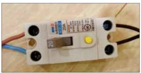
Use an ELCB (Earth leakage circuit breaker) for safety; long-time running can cause overheating
