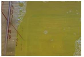
Water has to be clear after mixing. Soft water, when mixed with JWA and JS, will remain clear and have good foam. This indicates a good quality pesticide. Bubbles are the key in pesticide
