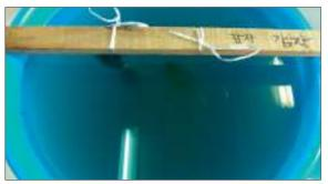
**4**.As microbes feed on potatoes and sea salt, bubbles start to rise. (Picture taken after 21 hours)
