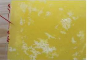
Clotting means problem. If water is not good, clotting can happen. You must change to soft water. Rainwater is typical soft water. If you use this clotted pesticide, you will have bad results – and many blocked nozzles.
