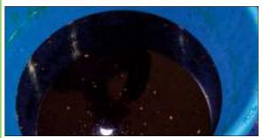
. Sulfur has melted completely. Sulfur content is 40%. If you leave it as is, crystals will form when cold.
