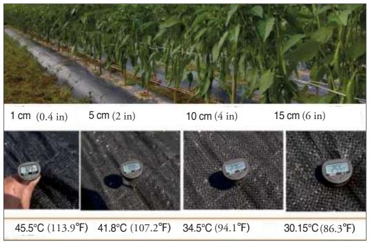
Temperature measured at the same time on the same day for weed mats (above). Compared to the plastic (below), temperature rise was much smaller in weed mats. Weed mats have small holes that allow the passage of air; hot air does not stay. It is UV-coated and can be used for 5 years
