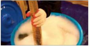
. In cold weathers, lumps tend to sink to the bottom; stir thoroughly including the bottom
