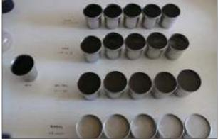
Add water in cups; add same amount of molasses in each cup; add a few drops of leaf mold water to inoculate the microbes. Cup on left has not added any germicide. Cups on right have been added with varying dose of germicide.
