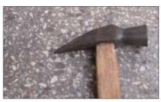
2. Use the sharp tip of a hammer to punch holes
