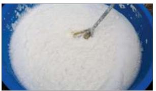
This is what happens when you over-drill with too little water. If water is not enough, JWA will not melt in water even if you mix with electric drill for a long time. JWA turned into a texture like white cream. Add water up to 3 cm (1.2 in) below the top and wait 2-3 days for bubbles to settle down. Clear JWA will gather below. If the white creamish film does not go away, remove it and use.
