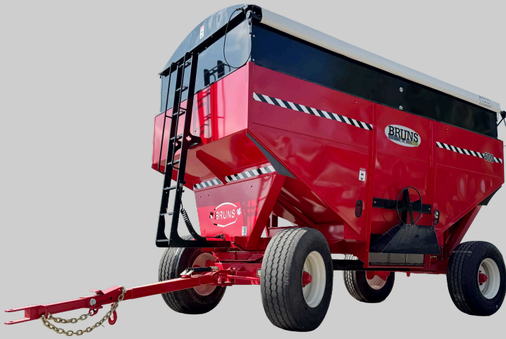
Shown with Horst 20 ton running gear, 425 tires
