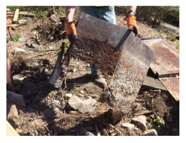
Corroded steel removed from center pier
