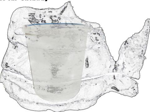
There were a couple of printer malfunctions that helped me achieve imprecise construction. For one thing, the machine tried to make a layer where there was no directive to do so. Then, it truncated the legs.
