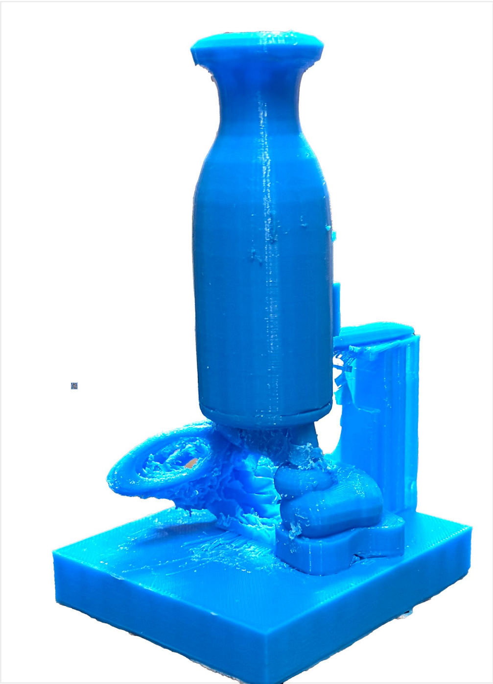
The Chromosome strands are filled with supports in the early stages of the print. These supports must be removed without breaking the strands.
