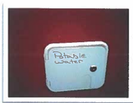
Potable Water Inlet
