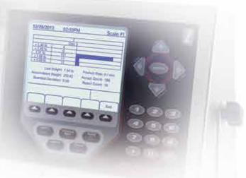
The statistics screen shows real-time monitoring of five pre-programmed weight zones, both per unit and cumulatively, illustrating where product falls within a targeted weight range.
