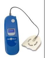
\*PainShield is a personal use 90kHz surface acoustic wave ultrasound device.
