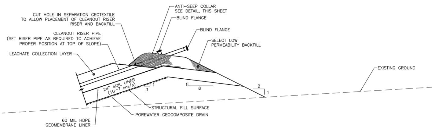
**CLEANOUT RISER AT TOP OF SLOPE**
