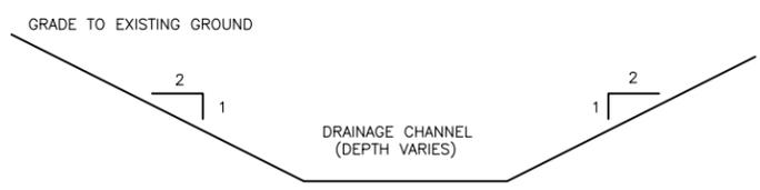
**PERIMETER DRAINAGE CHANNEL DETAIL**
