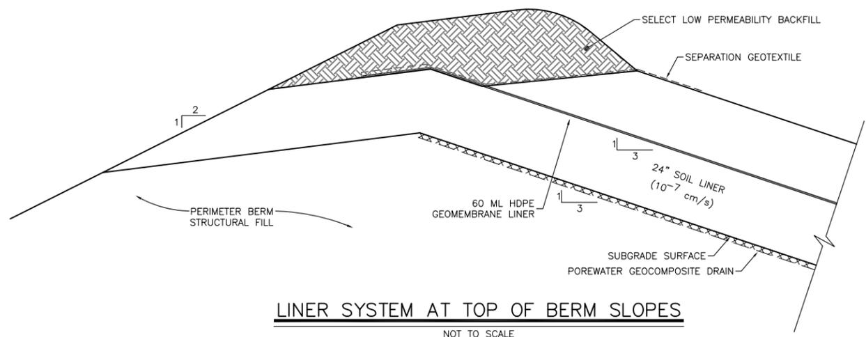
**LINER SYSTEM AT TOP OF BERM SLOPES**
