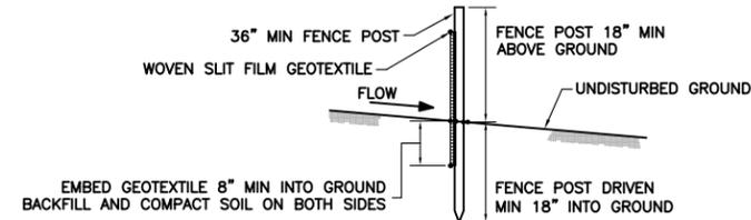
**SILT FENCE SCHEMATIC DETAILS**
