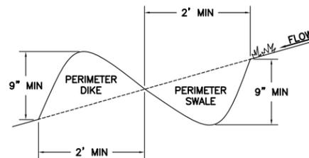
**PERIMETER DIKE SCHEMATIC DETAIL**
