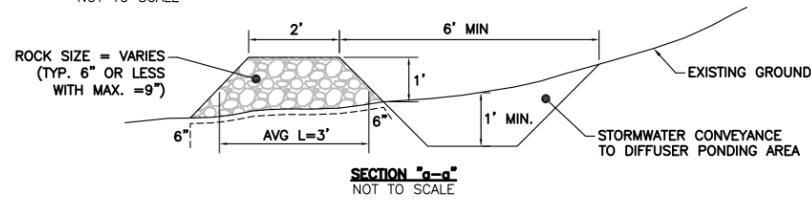
**FLOW DIFFUSER SCHEMATIC DETAIL**
