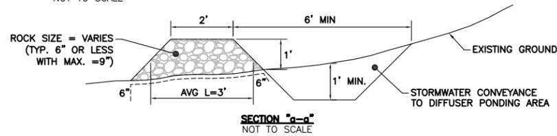
**FLOW DIFFUSER SCHEMATIC DETAIL**
