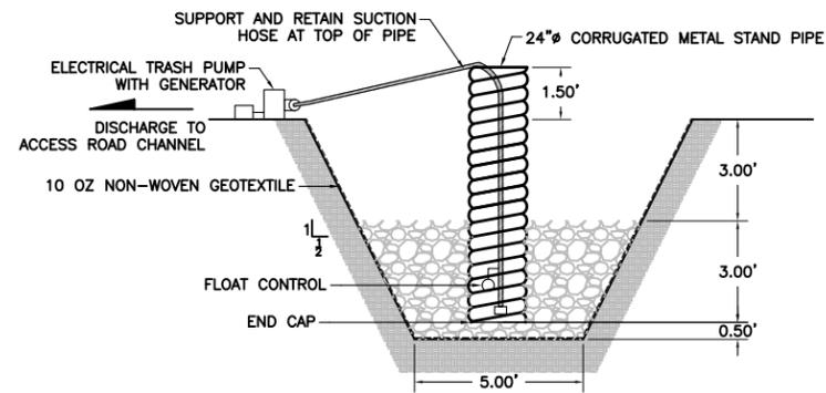
**SUMP PIT SCHEMATIC DETAIL**
