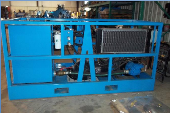
Diesel Hydraulic Power Unit
