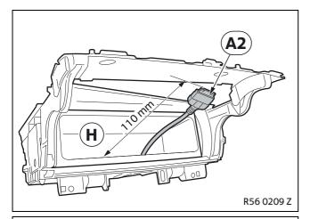
Pull branch **A2** out of the iPod interface storage tray **H** as far as dimension shown.
