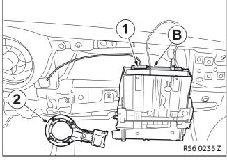
On cars with SA 694 (CD changer preparation), the tied-back CD changer plug (1) must be released and the shorting plug (2) removed. ◀
