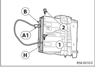
Attach CD changer/storage tray holder (1) to iPod interface storage tray **H** using screws previously removed (2).
