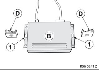
Fit speed nuts **D** to extended holes (1) on the interface **B**.
