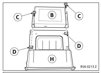
Fit speed nuts **D** to iPod interface storage tray **H**.
