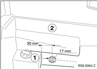
Drill a hole (1) in the glove compartment (2) using a 17 mm step drill bit according to the dimensions shown.
