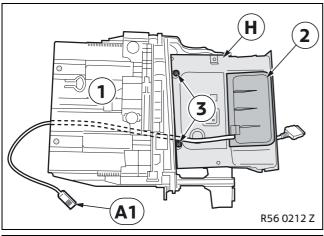
Remove screws (3) from iPod interface storage tray **H** (required later).
