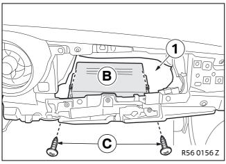
Attach interface **B** to the glove box (1) using self-tapping screws **C**.
