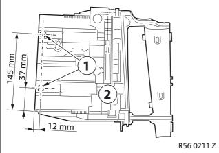
Mark the holes (1) according to the dimensions shown on the CD changer/storage tray holder (2) and drill through with a 5 mm twist drill bit.
