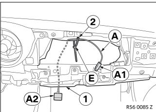
Pull branch **A1** of the connection cable **A** inwards until iPod connection plug **A2** is just above the outer edge (1) of the glovebox.
