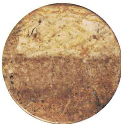
Cored section of low grade gold ore from the Mohave Desert of California. This rather unspectacular rock is rhyolite tuff breccia, and the microscopic gold which it contains can be detected only in an assay laboratory. Large volumes of such low grade ore form the foundation for modern western gold mining. (Core diameter is approximately 3 inches.)
