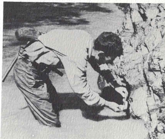
Geologist reading amount of dip of strata. The instrument is a Brunton Compass.
