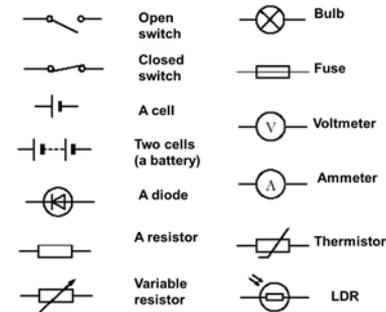
A **switch** turns a circuit **on** and **off**, by closing or opening a gap in a circuit.
