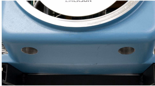
Figure 2-6: Wiring Entries on the Under Side of the Lower Enclosure
