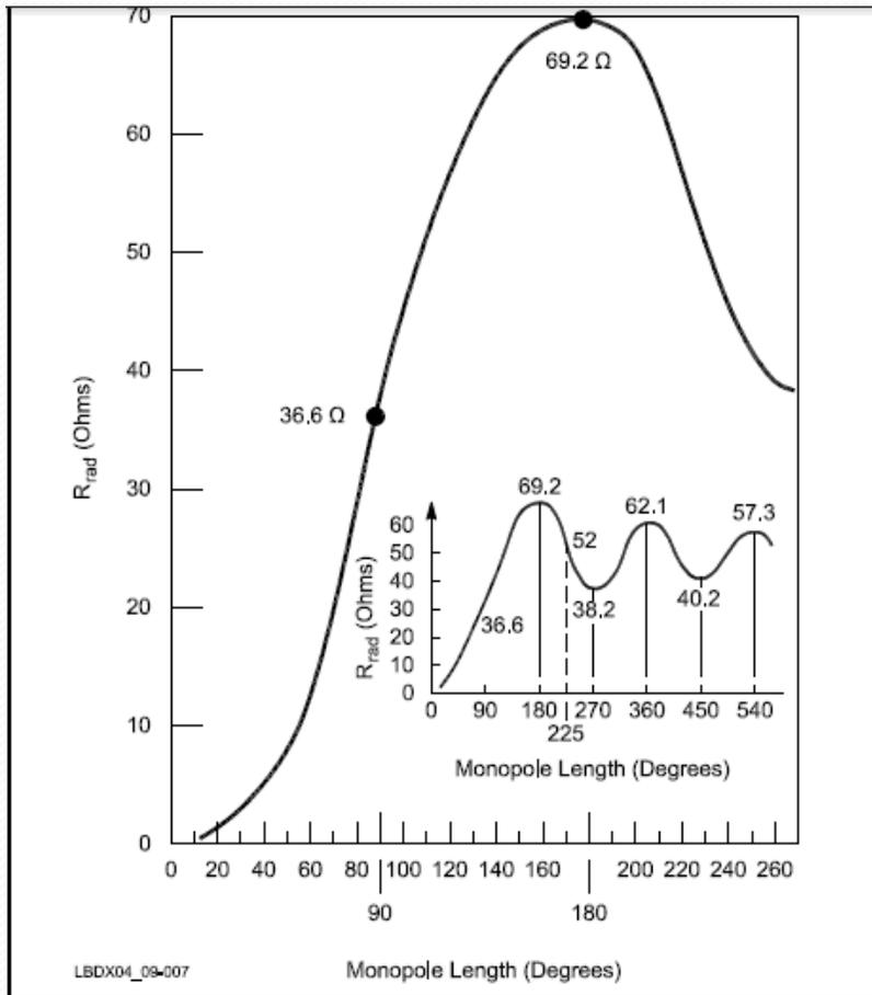
Figure 2.29 — Radiation resistances (at the current maximum) of monopoles with sinusoidal current distribution. The chart can also be used for dipoles, but all values must be doubled.
