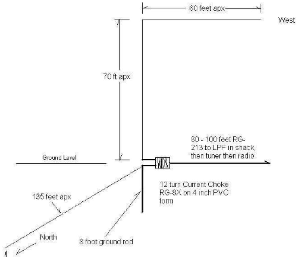
Single Radial, insulated 14 g housewire, laying on the ground.
