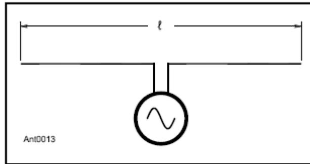
**Figure 2.1 — The center-fed dipole antenna. It is assumed that the source of power is directly at the antenna feed point, with no intervening transmission line. Although  $\lambda/2$  is the most common length for amateur dipoles, the length of a dipole antenna can be any fraction of a wavelength.**
