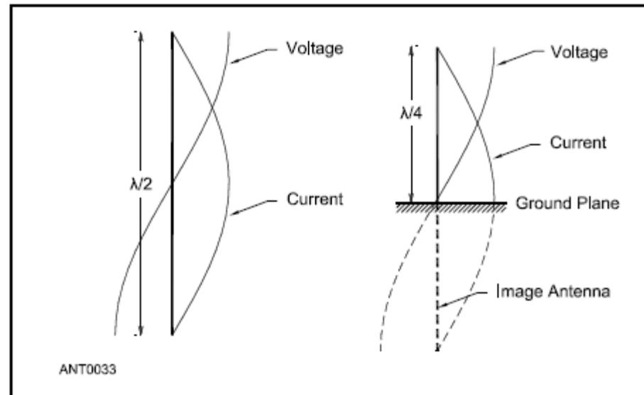
**Figure 2.25** — The  $\lambda/2$  dipole antenna and its  $\lambda/4$  ground-plane counterpart. The “missing” quarter wavelength is supplied as an image in “perfect” (that is, high-conductivity) ground.
