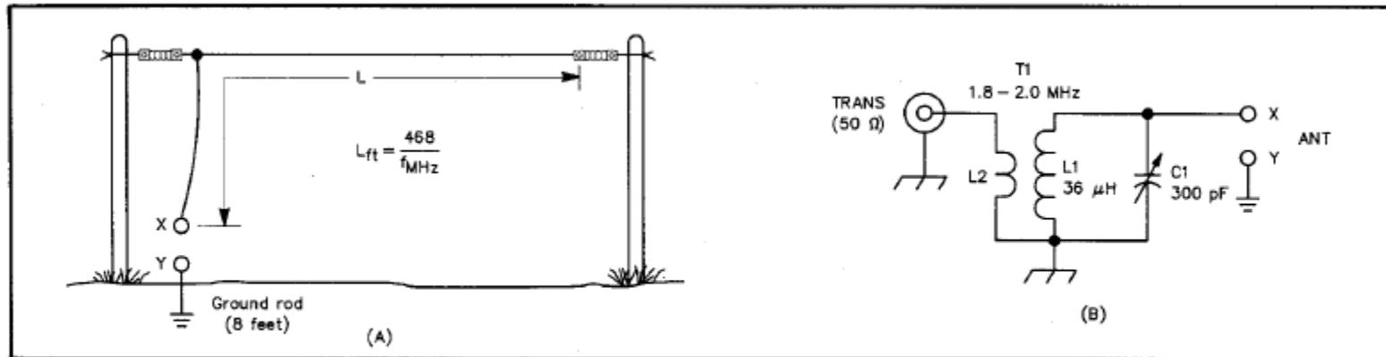
Fig 2—A  $\frac{1}{2}$ - $\lambda$  version of the antenna in Fig 1. This antenna is similar to one used at W4ZCB. L1 may have a relay-selected tap to permit operation on 80 meters as well. L1 and C1 are outside the house at the antenna feed point in a weatherproof box. C1 is motor driven and should have wide spacing or be a vacuum variable capacitor. Illustration B shows a suitable matching network.
