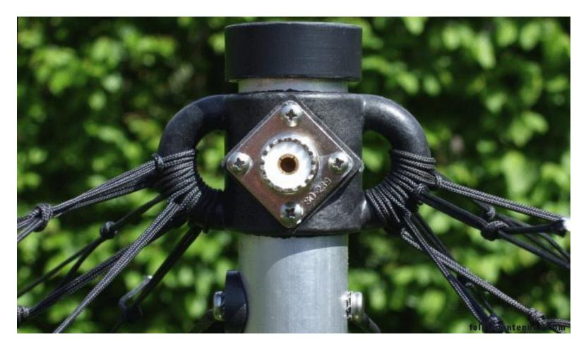
The hub takes up six swivel spreaders and electrically isolates the center post from the mast or rotator underneath
