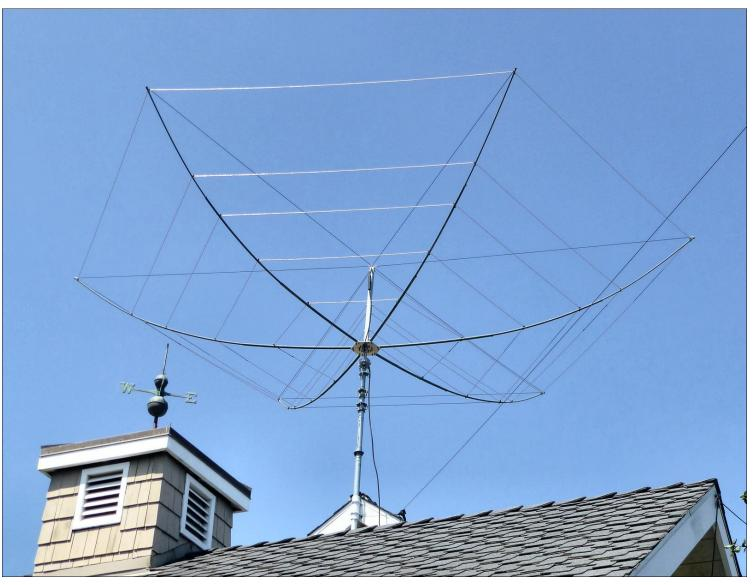
Because of the light weight and low wind load of a typical Hex Beam, a large tower (Rohn 25G and such) isn't needed.
